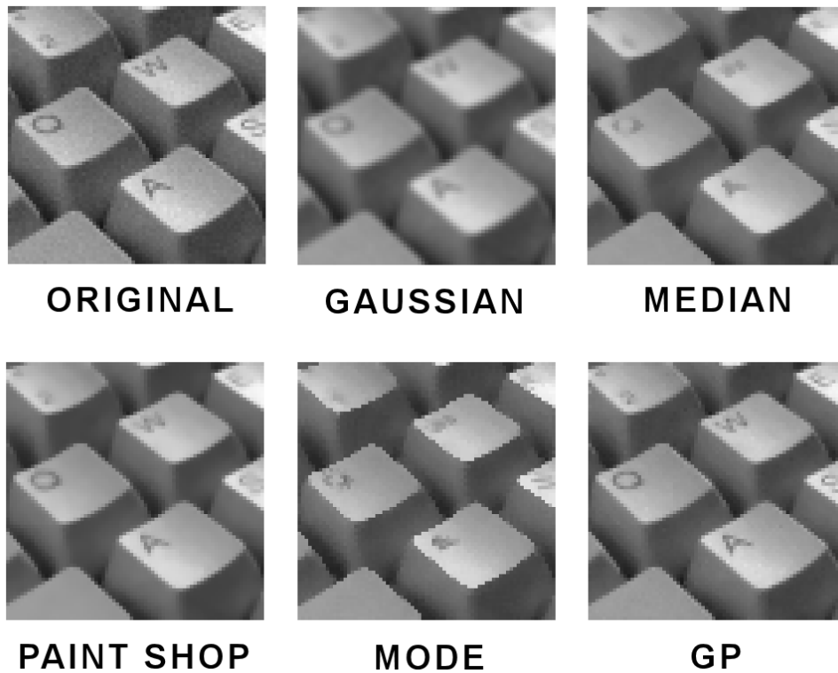
Figure 3.1: Different noise reduction techniques working on the original, noisy image. Gaussian filtering removes noise effectively but is too indiscriminate. Median filtering preserves more definition (although some is still lost). “Paint Shop” refers to the edge preserving smooth option in Corel Paint Shop Pro X2®. The author’s implementation of a Mode noise filter causes a slight sharpening effect. Finally, the results from a noise filter evolved by the author’s GP toolkit.
