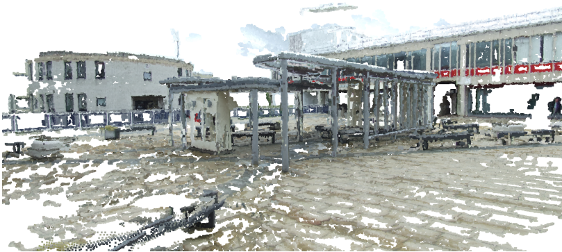
Figure 9.9: Views of a reconstruction of Square 2 using a structure from motion technique
