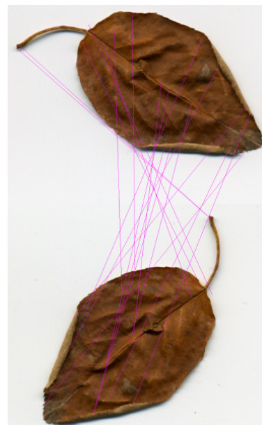
Figure 7.16: An example of feature matching using SIFT
